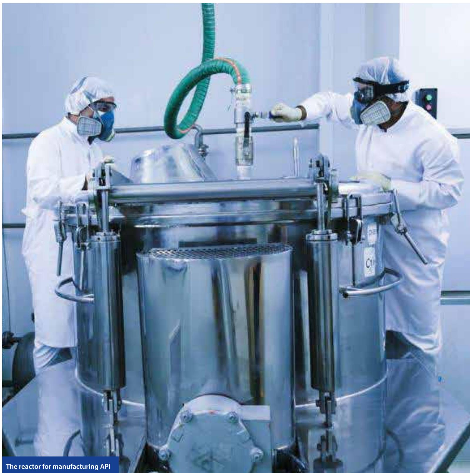
The reactor for manufacturing API
